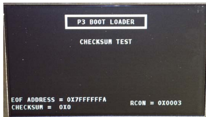
P3 programmed with the wrong firmware boot code
