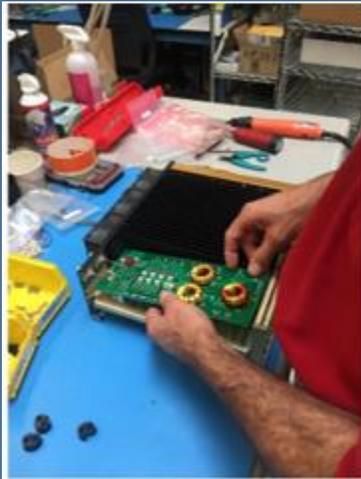
**Installing the Antenna Tuner**
