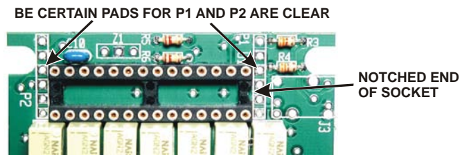
Figure 6. Installing Socket for U1.
