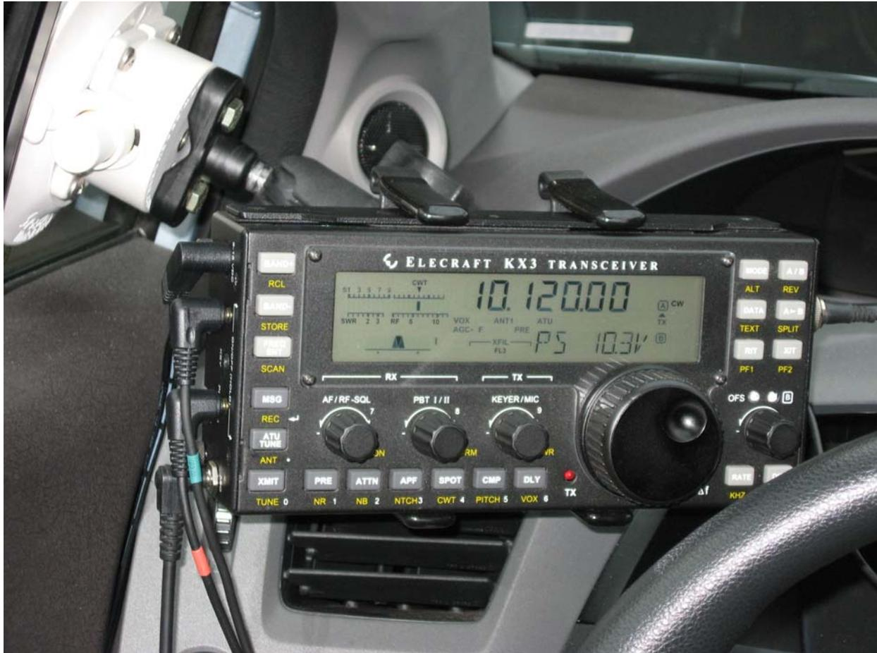
Figure 2. Seasucker 6018 vacuum mount with a KX3 in a Honda Civic. Note the use of the Elecraft KX3-PCKT cable set on the left. The right angle arrangement keeps cable layout tidy and out of the way. Below the audio cables (left side), a retaining clip is used to keep the bundle together.
