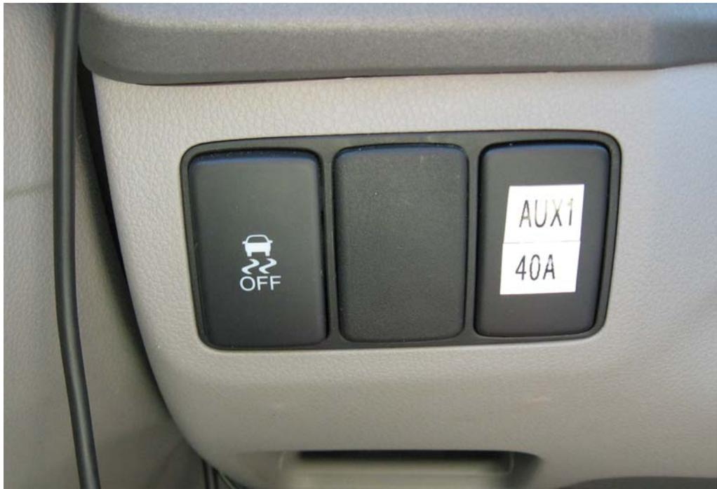
Figure 5. 40A branch circuit switch on the Civic's instrument panel. There were two "dummies" in this panel, so I removed the rightmost one and filled its slot with a Honda standard panel switch replacement. The KX3 and mount aren't seen, but they are located directly above this panel. The microphone cable is shown hanging at the left.
