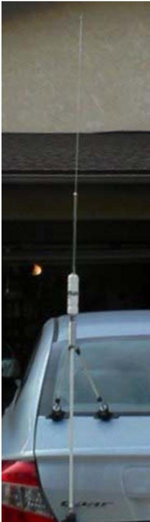
Figure 9. Trunk lip-mounted Hustler short mast with a 40m resonator attached.
