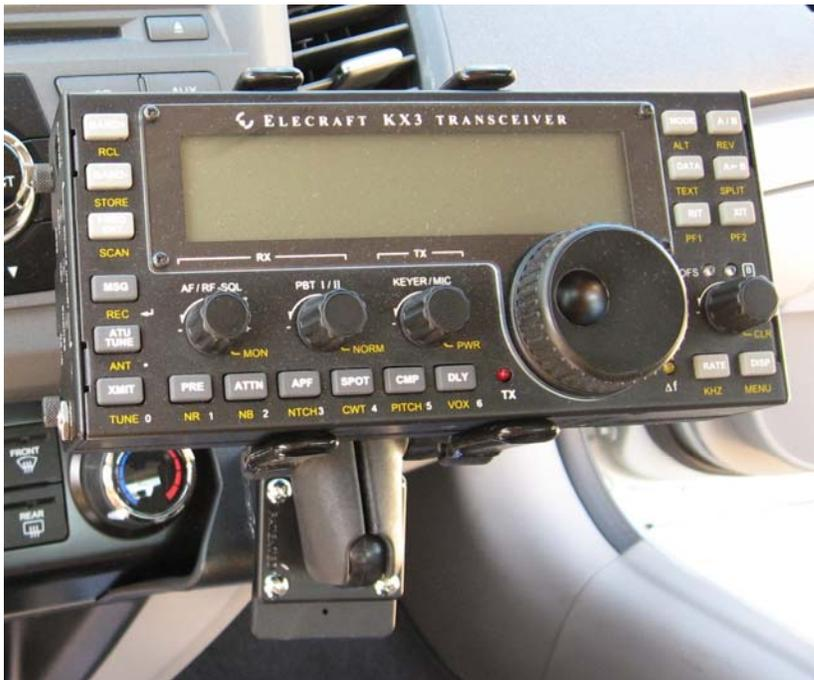
Figure 1. ProClip dashboard mount in a 2012 Honda Civic supporting a RAM double-arm clamp from an AMPS 1" ball adapter. The cradle retaining the KX3 is the same unit as shown in Figure 2 (also made by National Products – tradename: RAM).
