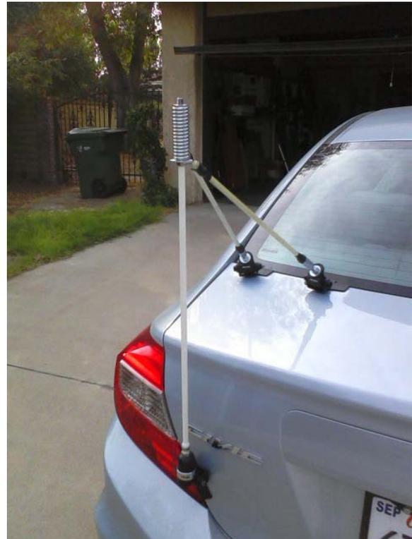
Figure 10. Detail shot of the tripod mount and the Hustler short mast.
