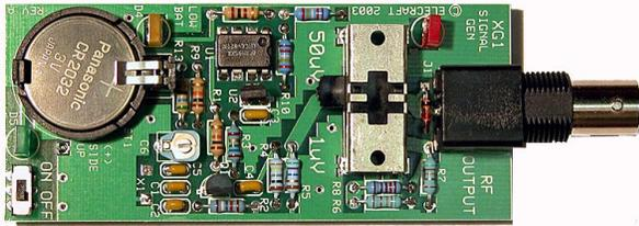
**XG1& XG2 Receiver Test Oscillators / S-Meter Calibrator**
