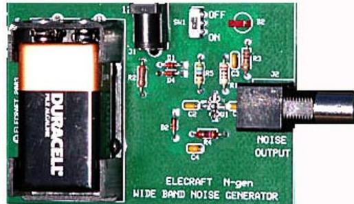
**N-gen Wideband Noise Generator (100 kHz - 500 MHz)**
