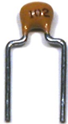
Figure 12. Forming Capacitor Leads.
