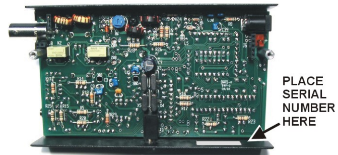
Figure 28. Installing Serial Number Label.
