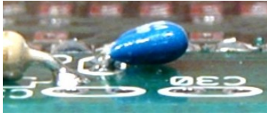
Figure 6. Positioning C39 Against the PCB.
