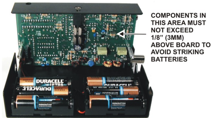
Figure 29. Checking Component Clearance.
