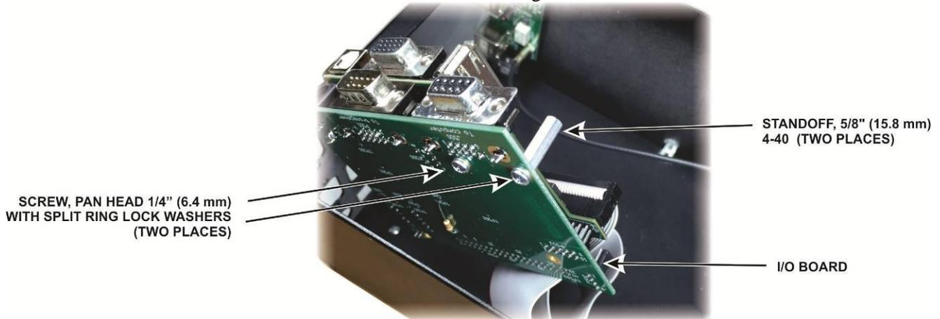
Figure 3. Installing Standoffs on P3 I/O Board.
