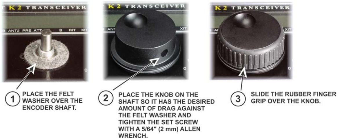
Figure 4. Installing the Main Tuning Knob.
