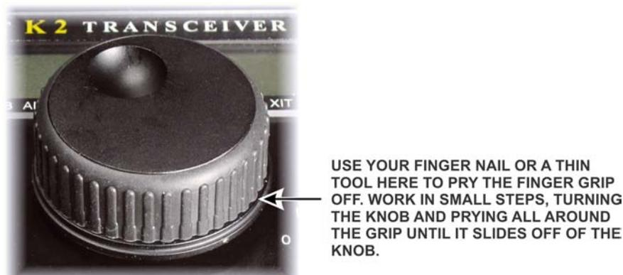
Figure 5. Removing the Finger Grip.
