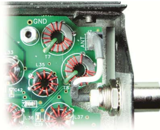
Figure 6. Connecting the Antenna Plug to the RF Board - No KXAT3 Installed.
