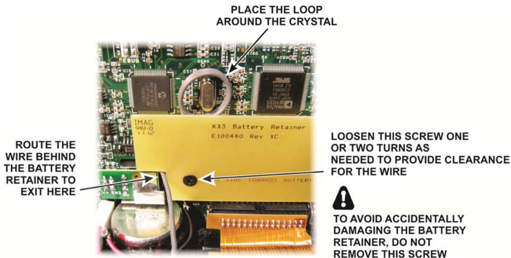
Figure 3. Positioning the Test Antenna at the 16 MHz Oscillator.
