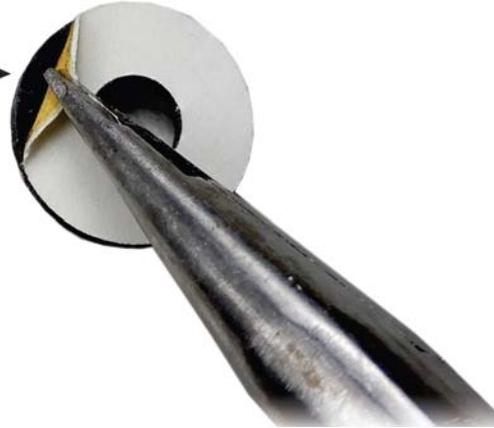
Place the washer on the VFO B encoder as shown below.
