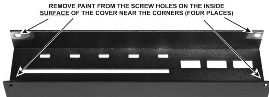
Figure 9. Preparing Front Panel Cover for Mounting
