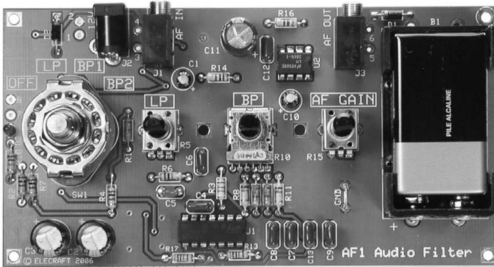
Figure 1. Assembled Audio Filter.
