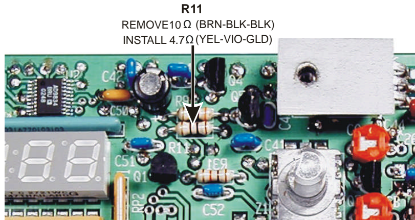
Figure 1. Replacing R11.
