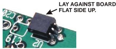
**Figure 13. Installing U2 on the Control Board.**
