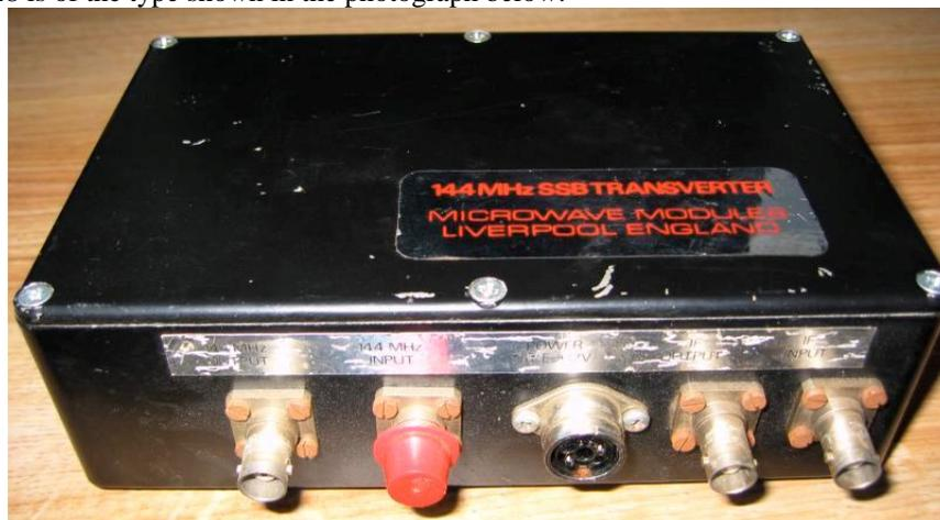
The red cap covers a socket marked “144 MHz Input” which is not generally used in these transverters.
