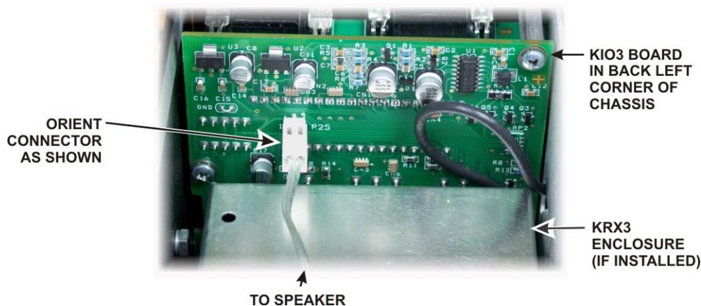
**Figure 6. Connecting the Speaker Cable.**
