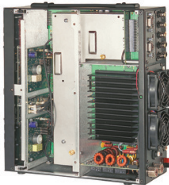
Figure 5 — Interior view of the K3/100. The 100 W output stage is shown in the center rear. The subreceiver occupies the L shaped enclosure filling the front portion of the inside of the radio. Removing the two knurled nuts and three miniature coax connections allows the subreceiver to be easily removed to add main receiver roofing filters, for example.
