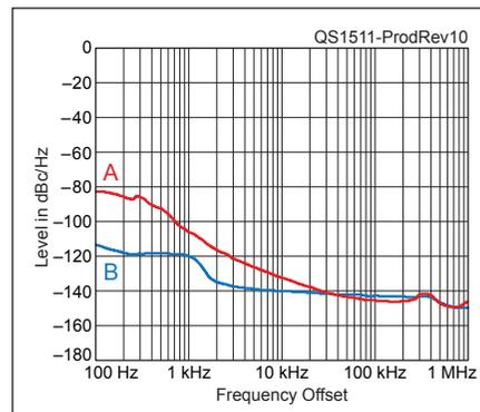
**Figure 10** — Spectral display of the Elecraft K3 transmitter output during phase noise testing. Power output is 100 W on the 14 MHz band with the original synthesizer (line A) and after the synthesizer upgrade (line B). The carrier, off the left edge of the plot, is not shown. This plot shows composite transmitted noise 100 Hz to 1 MHz from the carrier. The reference level is 0 dBc, and the vertical scale is in dBc/Hz.
