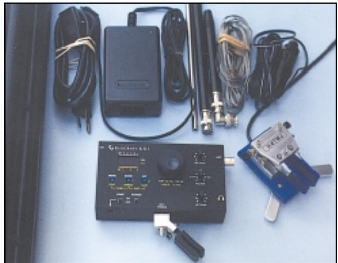
*Photo 6— Our “minimalist” gear laid out for the QRP road trip. Items include the Elecraft KX1 with optional case-mount paddle, external “Parkwood” paddle from WB9LPU ([wb9lpu@earthlink.net](mailto:wb9lpu@earthlink.net)), MFJ AC power supply, Maldol pull-up antenna with clip-on counterpoise, and self-supporting “Buddipole” antenna. Mobile antennas are not shown.*
