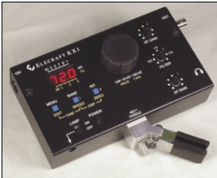
Photo 1— Equipped with all its options, Elecraft's new KX1 is a three-band CW transceiver with built-in battery pack, automatic antenna tuner, electronic keyer and paddle, LED, plus Morse code readouts and even a logging light. The little rig is microprocessor controlled with a superb receiver, 4-watt transmitter, and silky smooth break-in operation. (Photo courtesy Elecraft)
