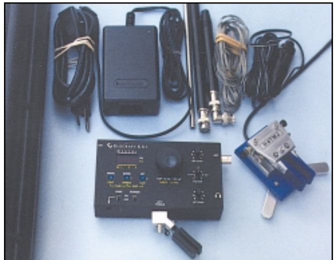
Photo 6— Our “minimalist” gear laid out for the QRP road trip. Items include the Elecraft KX1 with optional case-mount paddle, external “Parkwood” paddle from WB9LPU ( wb9lpu@earthlink.net ), MFJ AC power supply, Maldol pull-up antenna with clip-on counterpoise, and self-supporting “Buddipole” antenna. Mobile antennas are not shown.
