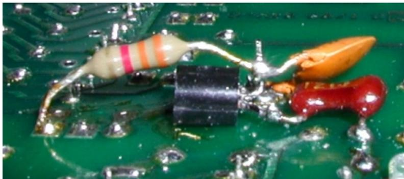
Photo #3 - Mod showing transistor BASE lead bent AWAY from RF board
